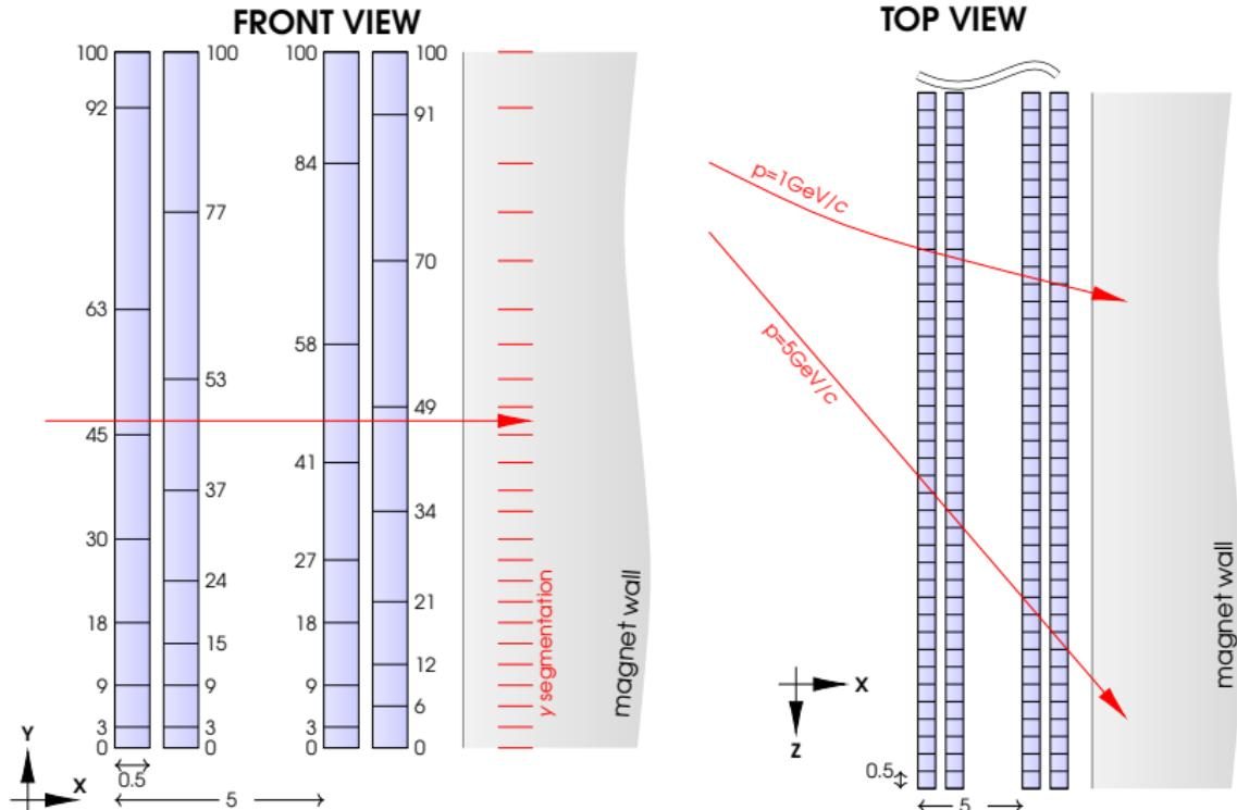
Not in scale, numbers are panel coordinates and sizes in cm. Crossing particles are represented as red arrows.
