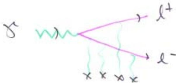
$$\sigma = \frac{28}{9} \frac{\alpha (Z\alpha)^2}{m_e^2} \left[ \log \frac{2\nu}{m_e} - \frac{109}{42} - f(Z\alpha) \right]$$
