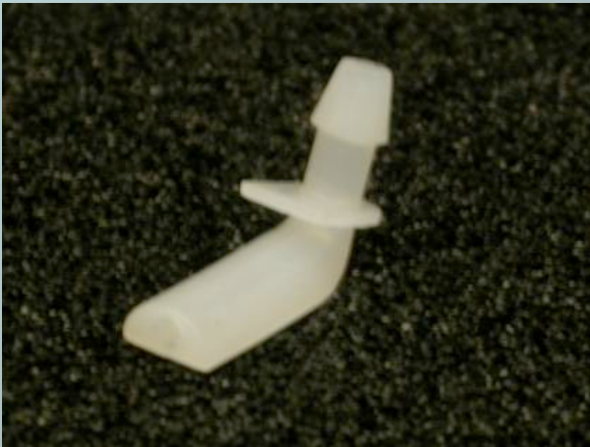
Barbed fitting glued to ends of carbon fiber heat sink
