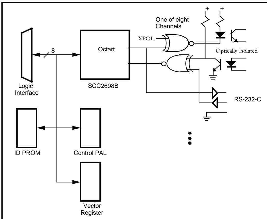
**Figure 1 Block Diagram of IP-Octal Opto Serial**
