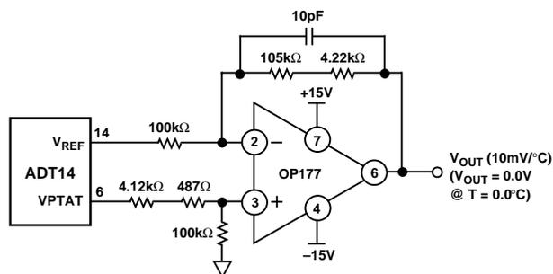
Figure 26. Translating 5 mV/K to 10 mV/°C
