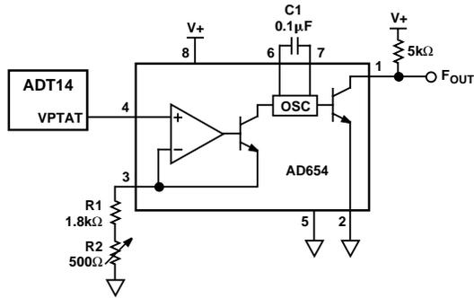
Figure 23. Temperature-to-Frequency Converter
