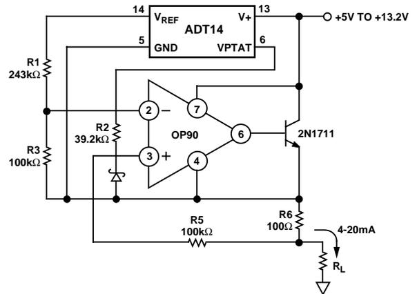
Figure 22. 4 mA to 20 mA Current Loop
