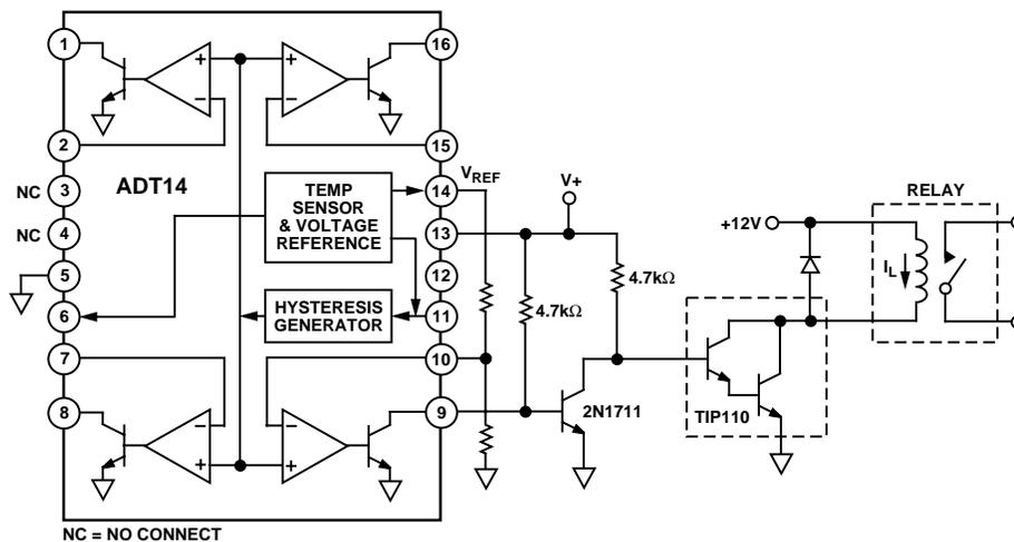
Figure 19c. Darlington Transistor Can Handle Large Currents
