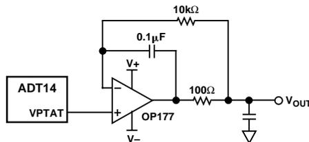
Figure 20. Buffer VPTAT to Handle Difficult Loads
