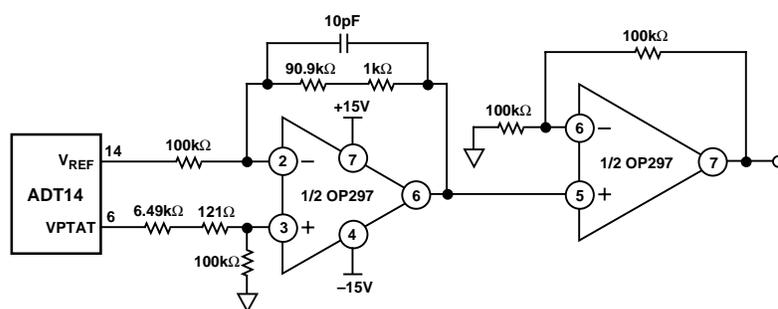
Figure 27. Translating 5 mV/K to 10 mV/°F
